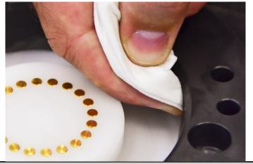
Clean the cavities of the locking balls with a lint free
