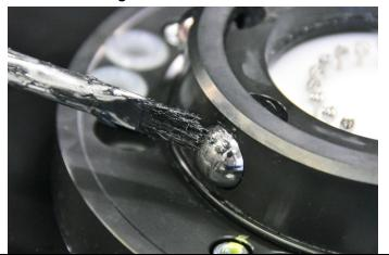
Apply a small amount of grease (Molykote BR2Plus) on the locking balls.
