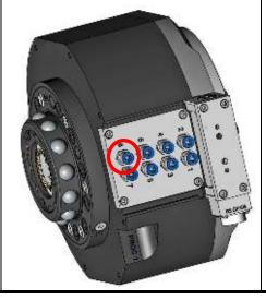
Connect compressed air to the air connection marked OPEN. Exhaust air is evacuated via connection marked CLOSE.
