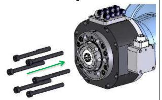
Mount the swivel tool changer with the enclosed screws. Use a torque wrench when tightening (see tightening torques above).
