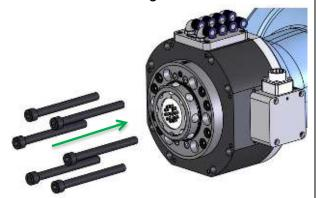
Mount the swivel tool changer with the enclosed screws. Use a torque wrench when tightening (see tightening torques above).
