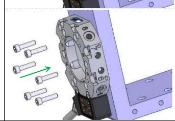
**NOTE!** For TA100 fastening screws can only be entered from the tool attachment side.
