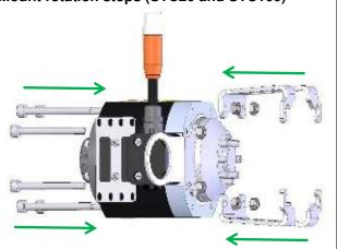
Mount the rotation stops with enclosed screws and nuts. The tightening torque for STC20 is 4 Nm, and for STC100 it is 6 Nm.
