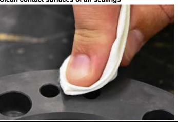
Wipe the contact surfaces of the air sealings clean with a lint free cloth.
