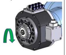
Rotate axis 6 to put the rotation stop in position for mounting.
