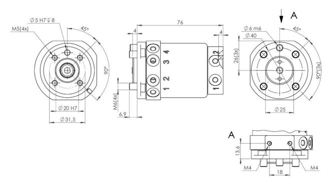
Swivel S20-6 transfers 6 pneumatic channels to the tool.
