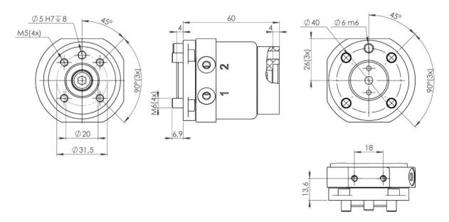
Swivel S5-4 Ø40 transfers 2 pneumatic channels to the tool.
