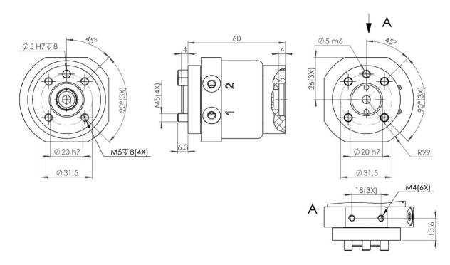
Swivel S5-2 Ø31 transfers 2 pneumatic channels to the tool.
